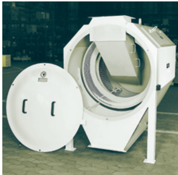
Inlet channel to the inside of the screening drum.
