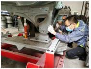
The cab straightening work platform 00201 is a solid, strong and stable work platform that can work efficiently and simplify cab maintenance operations. The official is composed of a sturdy base and a fixing kit. The base can be fixed on the I-beam track of the workshop or on the ground with the help of expansion bolts. The fixing kit is movable, which is conducive to the installation and fixation of the cab. Even the severely damaged cab is easy to fix.
