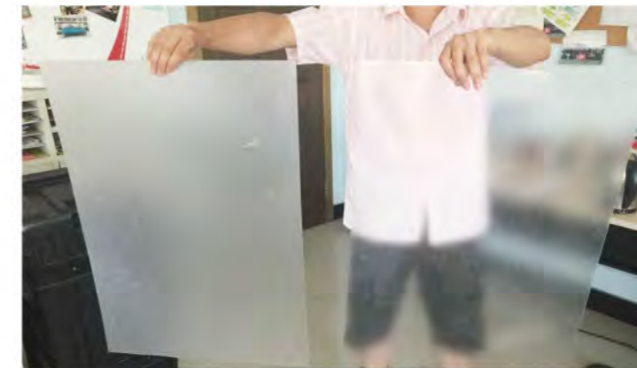
Frosted/ MATTE ← | → ANTI-GLARE/ANTI-REFLATION
