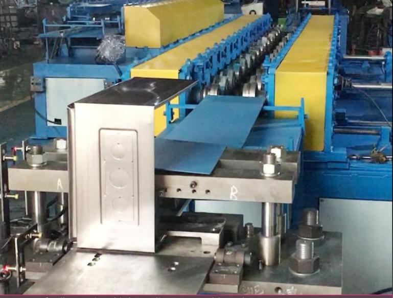
16 sets of roller station, high-quality Gr12 mold steel, HRC up to  $58 \sim 60^{\circ}$  are processed by precision CNC machine tools, precision is  $6 \sim 7$ , surface roughness is above 0.8, no scratches on the surface.
