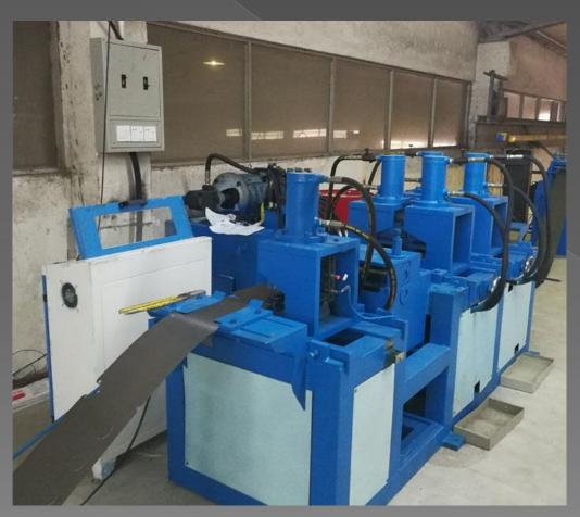
Servo feeder, Hydraulic Hole Punch 2KW servo system, precision feeder. Hydraulic punching device (tool)
