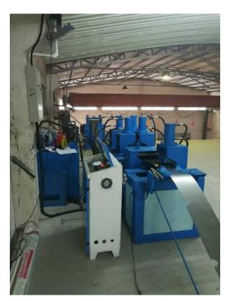
Roll forming machine system, The main machine base of this production line is welded with 100\*100\*3MM square steel, Shenzhen Superda
