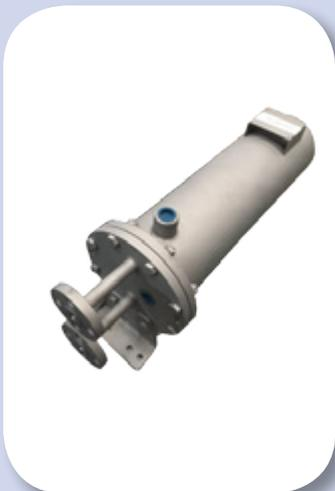
Plan 21 is a mechanical seal flushing system that uses the cooled pumping media as the flushing fluid. Plan 23 is a mechanical seal flushing system that creates a circulation for another flushing fluid in the seal flush chamber. The plan aims to prevent overheating and failure of seal face. Usually it is applied at the condition of media temperature higher than the mechanical seal limit temperature.
