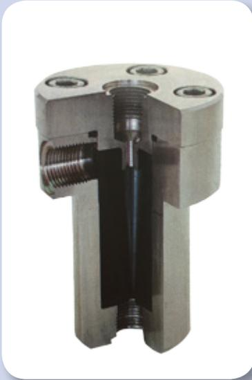
Plan 31 is a mechanical seal flushing system that uses filtered pumping media as the flushing fluid in the case of pumping media with abrasive particles. The media with abrasive particles at pump discharge first through the cyclone separator for particle centrifugal separation. The clean media liquid is piped to flush the mechanical seal, and the left media with particles is piped back to pump suction.
