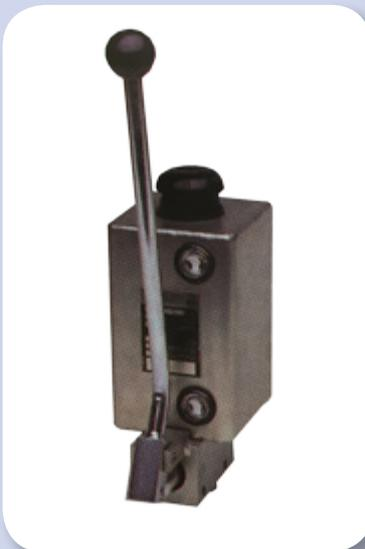
The Hand Refill Pump is applied in Plan 53A/53C systems in the purpose of filling the buffer liquid. Because Plan 53A/53C systems are used together with Arrangement 3 dual seals, the pressure inside the pressure reservoir is higher than the media side. Under this situation, a hand refill pump is required to refill the buffer liquid into the reservoir by manual pumping if the liquid level is too low.
