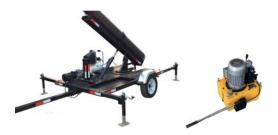
Hydraulic lifting system: 3 Tons hydraulic cylinder with 750W 220V/50Hz motor with support beam for mast tilt from horizontal to vertical and from vertical to horizontal (electric motor hydraulic unit with manual operation back up)
