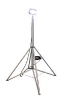
5m Manual Push Operation Telescopic Mast Lighting Tower aluminum alloy materials manual push telescopic mast, 5m extended height, 5 sections, section dia. 33mm, 40mm, 47mm, 54mm
