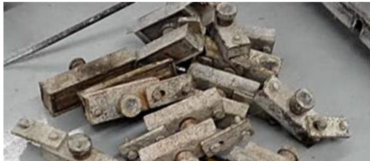
Magnet box deformation
