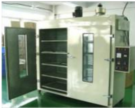
Unit modules aging furnace
