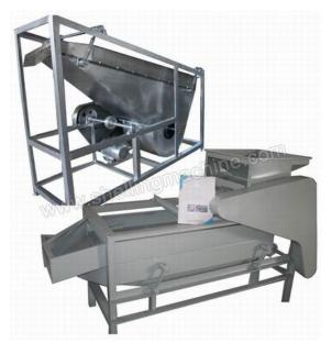
◆ Palm nuts kernel separating machine is available for separating nuts kernels from hard shells with the help of airflow.
