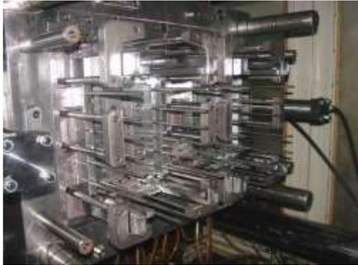
Precise injection mould
