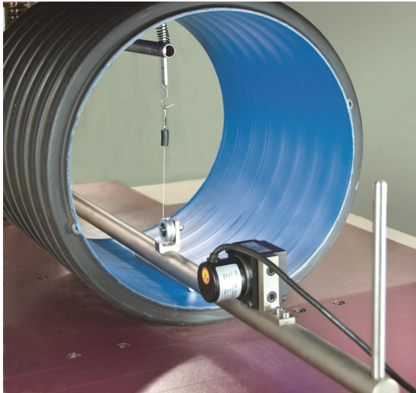
Inner diameter measurement system
