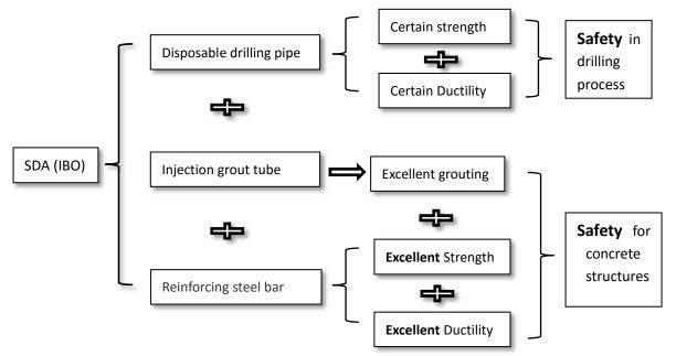
Note: SDA = Self Drilling Anchors, i.e. Hollow Bar Anchors, or Hollow Bar Soil Nails, Micropiles.
