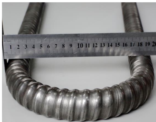
Bend test of a hollow bar anchor
