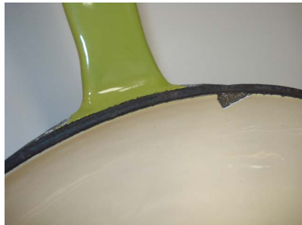
Picture 9: Enamelling on the inside chipped off
