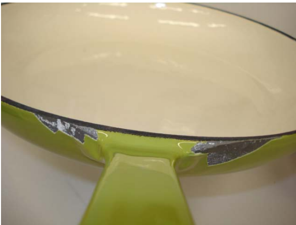
Picture 8: Enamelling on the outside chipped off
