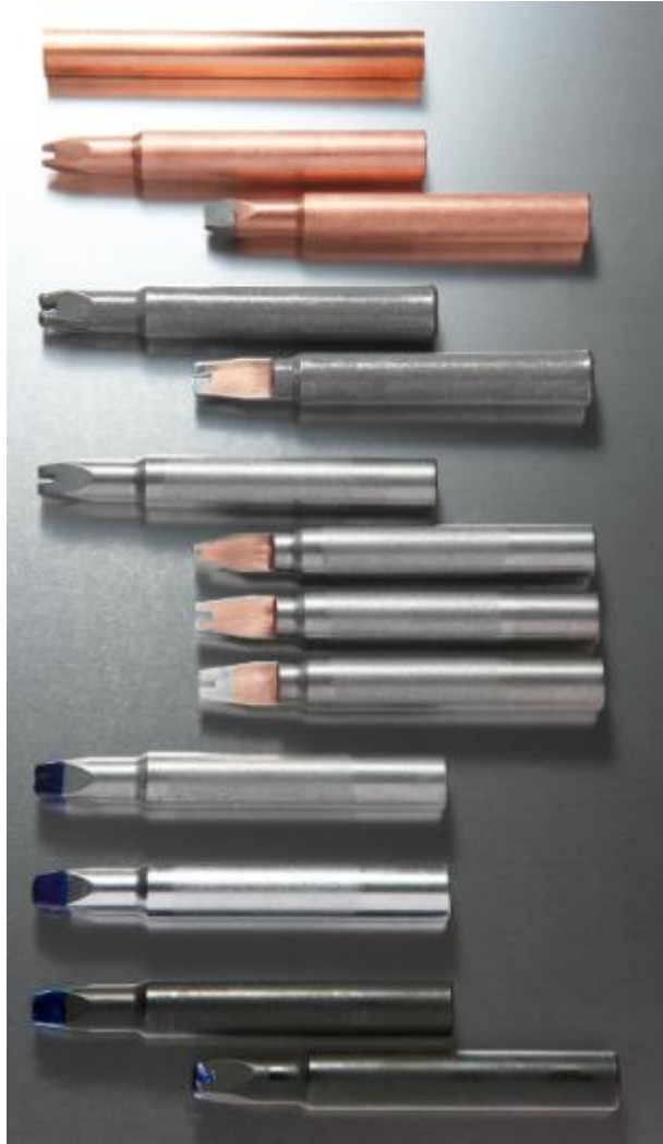
Copper to finished product
