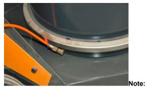
The compressed air must be free of oil and water!
