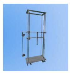
It's strictly designed according to IEC62262:2002-relates to IK ratings. It's applied to the mechanical impact strength test. And the impact angel is adjustable, and the device can be moved all around.
