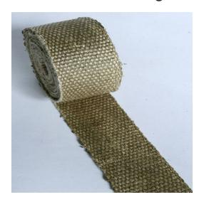
Vermiculite Coated Fiberglass Tape will withstand temperatures of 1500°F / 815°C continuous exposure. The base High Temperature fiberglass tape is fabricated from high quality type E fiberglass that will not burn.
