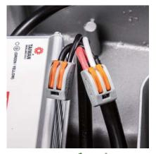
Utilize Germany **WALGE** connectors for output connections, safety, convenient and fast
