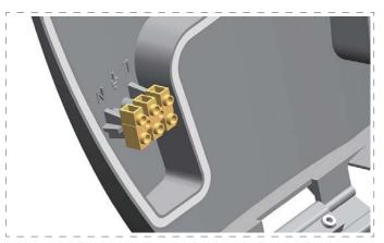
Connect the wires to terminal block accordance with L, N and  $GND \oplus$  on the cover of electrical box.
