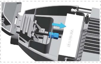
Thread the cable by M16 waterproof connector, do not tighten the connector.
