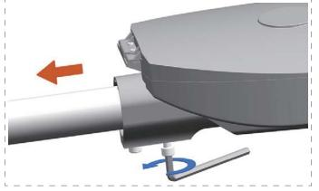
Mount the street light and adjust to proper position, fix the two M10 screws.
