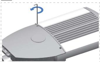
Open the electrical box by remove two M5 hexagon screws.
