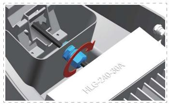
Tighten the waterproof connector after connection finished to avoid damage of pull.
