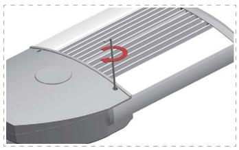
Close the cover, tighten the M5 hexagon screws both sides.
