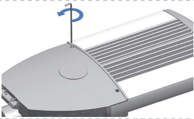
Open the electrical box by remove two M5 hexagon screws.
