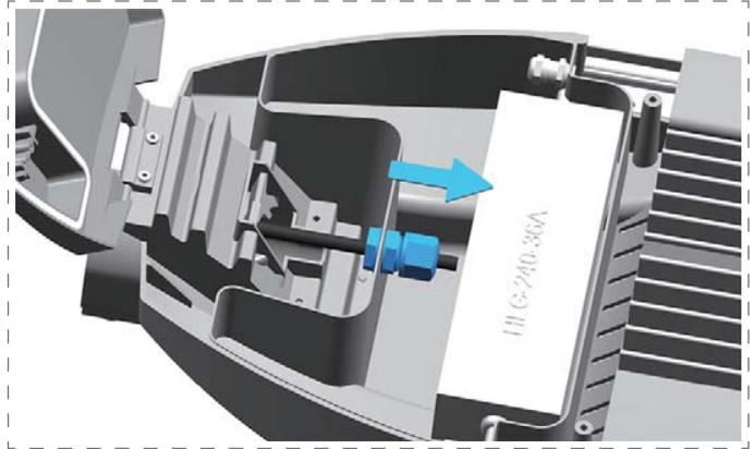
Thread the cable by M16 waterproof connector, do not tighten the connector.
