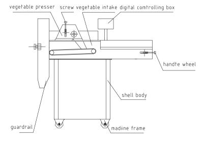
2.2 The vegetable intake part's frame, presser, bottom of shell body shell body's guardrail and machine's guaedrail are made of stainless steel. The transport belt is made of innoxious plastic, It's heath and safe.
