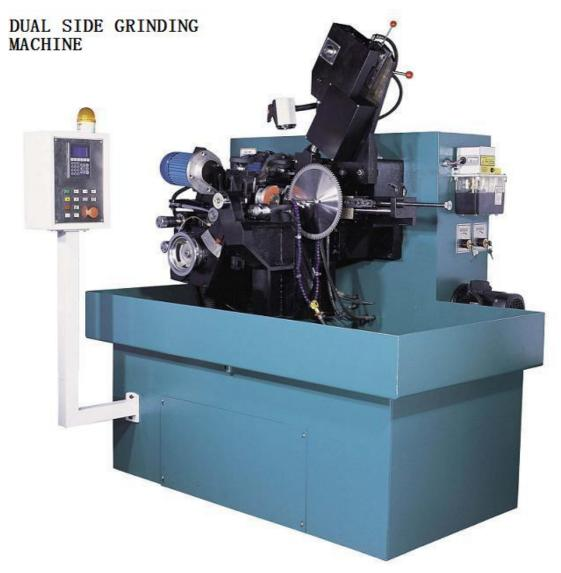
\*Machine tools of this type grind the two side angle at the same time, avoid the error caused by the different force, high precision and efficiency. They are suitable for batch process. Several machine tools can be operated simultaneously by one person.
