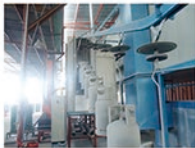
LPG tank powder coating line
