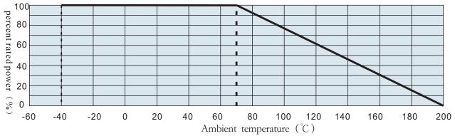
For resistors operated at an ambient temperature of 70°C or above, the power rating should be derated in accordance with the above derating curve.
