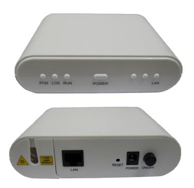
XDK-E8010U-B type ONU products fully comply with IEEE 802.3-2005 and the China Telecom EPON device technical specification (V2.1). It is operative, manageable and maintainable at telecommunication level, and can provide high speed data service for customers. It has a PON uplink port that connects to office end apparatus through optical fiber.
