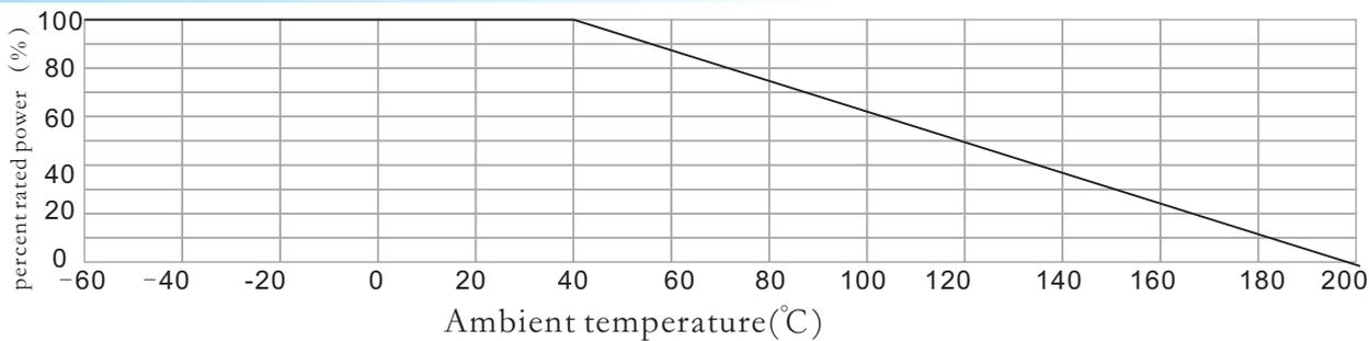
For resistors operated at an ambient temperature of 40°C or above, a power rating shall be derated in accordance with the above derating curve.
