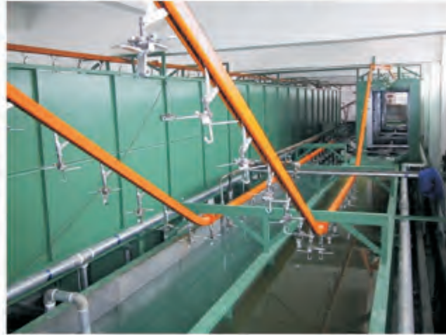
In-line dip washer with conveyerized system
