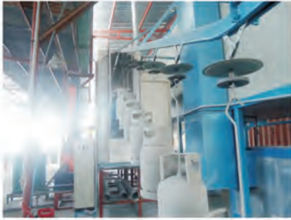
LPG tank powder coating line
