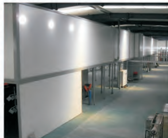
Tunnel type powder coating curing oven
