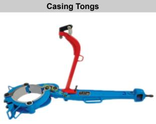
The 13-3/8 inch casing manual tongs is capable of making up or breaking out of the screws of casing and casing couplings of 14-3/8 in drilling operation, the rated load of it is 8KN.m(5,900 lb·ft)
