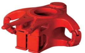
The TA Style Elevators are for use on tubing, casing and drill collars. The elevators are balanced for easy handling with safety lock and latch and guarded operating handles. Sizes range from 35 tons to 150 tons and cover all size tubular up to  $11^{1}/_{4}$ ".
