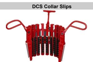
There are three types of DCS Drill Collar Slips: S, R and L. They can accommodate drill collars from 3in(76.2mm) to 14in(355.6mm) O.D.. The handling sizes can be adjusted by changing the quantity of inserts or slip body. They are designed and manufactured according to API Spec 7K.
