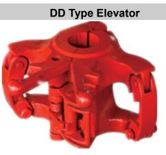
Model DD center latch elevator with square shoulder is suitable for handling drill collar, casing and tubing. The load ranges from 150 tons to 350 tons. The size ranges are from 2" to  $5^{1}/_{2}$ ".
