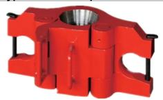
CDZ drilling pipe elevator is mainly used in the holding and hoisting of drilling pipe with 18 degree taper and tools in oil and natural gas drilling, well construction.CDZ drill pipe elevators are forged from high quality alloy steel, heat-treated, and NDT tested. The rated loads range from 150t (1350kN) to 500t (4500kN, and cover pipe sizes from 2.3/8" to 5.1/2" O.D.
