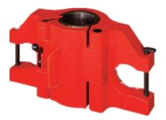
CD drill pipe elevators are conventional side door drill pipe elevators for handling 90 degree shoulder drill pipe in oil and gas drilling operation, CD drill pipe elevators are forged from high quality alloy steel, heat-treated, and NDT tested. The rated loads range from 150t to 750t, and cover pipe sizes from 2.3/8" to 9.7/8"O.D.
