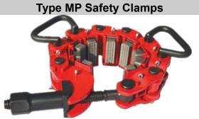
Safety Clamps Type MP are necessary tools for handling drill collars, flush joint pipes and small shoulder pipes. They could adjust pipes of different sizes by changing the quantity of chain links. They are designed and manufactured according to API Spec 7K.
