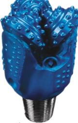
In addition to the features of MD motor bit, Mini MD slim hole bit is also designed with special bearing & seal structure and lubrication system. Mini MD bit's cutter material and cutting structure are reasonably matches with rock properties of the formation and this eliminated the specific problems such as low drilling efficiency and cutter breakage and loss, etc.
