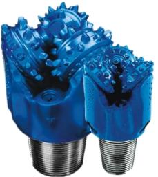
HA/HAT series bit adopts rubber seal with journal bearing, which can sustain higher WOB under normal rotary speed and is suitable for drilling in formations from very soft to middle hard properly selecting different cutting structure.
