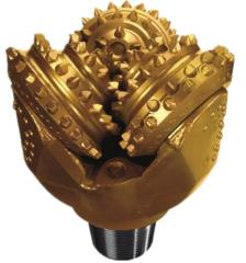
SKG series bit is designed with roller bearing and rubber O-ring seal. This bit can achieve longer footage and higher ROP when drilling under medium to low WOB and high RPM.
