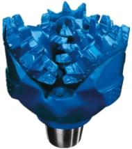
GA/GAT series bit adopts rubber seal with roller bearing, which is the ideal and economical tool for drilling applications where middle to low WOB and high RPM are required.
