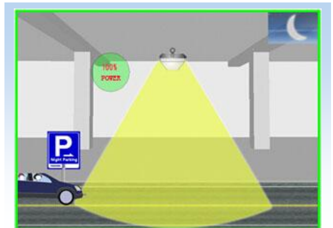
Model 2: When people enter the sensing area, all lights will turn on (100%)
