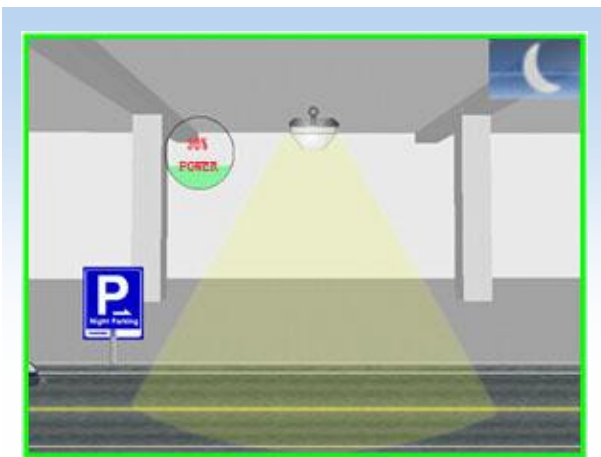
Model 1: Lights brightness keeps to be 30% (adjustable) when there is nobody
