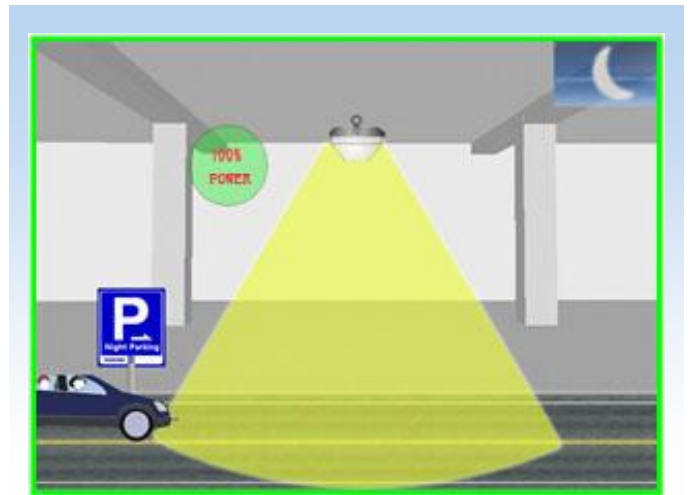
Model 2: When people enter the sensing area, all lights will turn on (100%)
