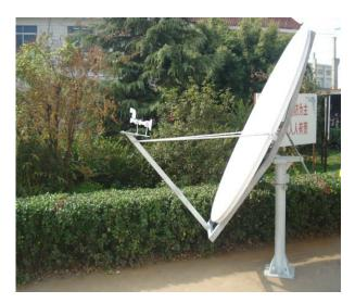
**Probecom 1.8Meter antenna** consists of two varieties, offset /ring focus antenna ,providing Tx/Rx 2-port feed in linear polarization, can offer superior Tx/Rx performance.
