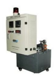
The dual-column double-position hydraulic screen changer is designed to work with two channels inside. It contains two screens that work at the same time: one screen works, while the other one is changed during the process of screen replacements, thus the replacement without machine halt is ensured and no interrupt of material fluid and of production will occur. Therefore, the screen changer meets the customers' requirement of higher productivity and better quality.
