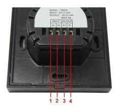
"1", "2": power input pins, input voltage range is 12-24V, "1" is negative pole, and "2" is positive pole.
