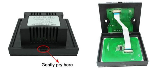
(2) remove the cable. Pull the locking of the terminal transposon, and then you can slowly remove the cable, as shown below:
