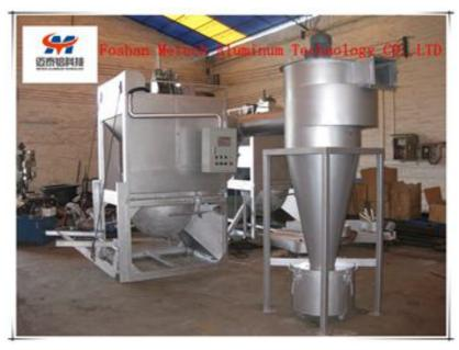
Hot Aluminium Dross Processing Machine (Aluminum Recovery System)
