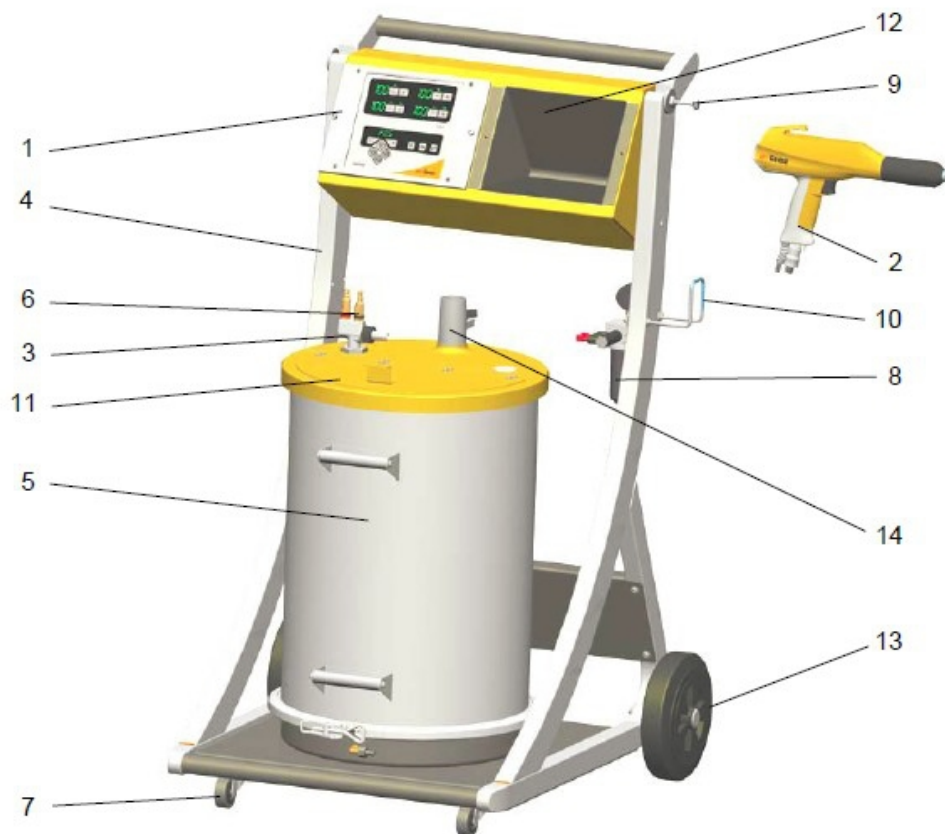
OptiFlex F manual coating equipment - structure
