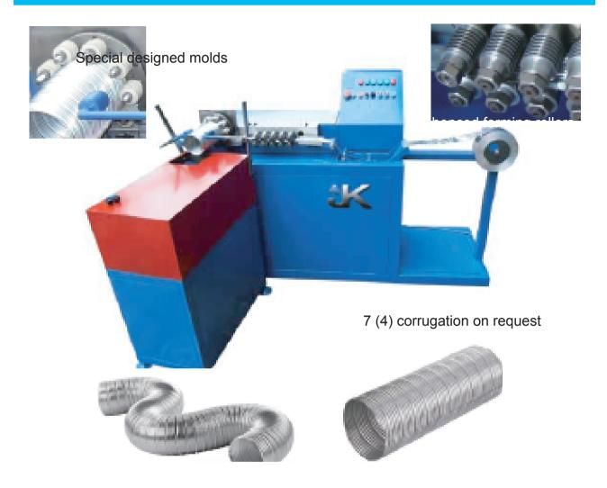
Aluminum tube is widely used in the kitchen, bathroom, air condition venting and HVAC system. The corrugated aluminum tube can easily compressed and strached, and the aluminum corrugat -ed tube can change its shape and keep it. The Auto cutting system is the most effecient.
