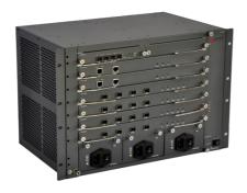
GX3700 is "GX3000" series GEPON OLT equipment with rack mount design. It provides 20 GEPON optical interfaces and connects 80 remote ONUs at most. It provides 4\*GE optical/electrical uplink interfaces. GX3700 with rack design is convenient for extending and upgrading service. GX3700 includes SW (switching control unit), GET (GE electrical unit)/GEO (GE optical unit), GEPON optical unit, fan unit and power supply unit.
