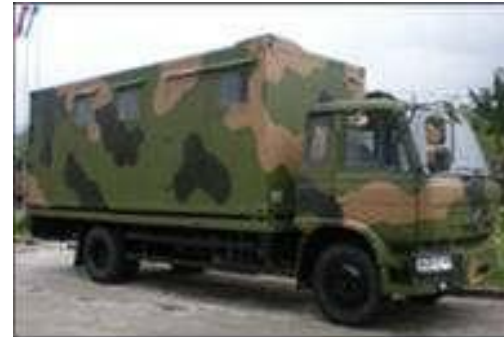
Military mobile power station
