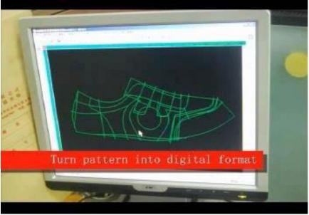
2.Design:Rapid design of the half pattern can be done through automatic edging and various edging, random arranged matrix, group sharing designation and analog layout of standard grap after extraction of the needed pattern sheet.
