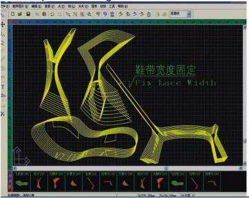
10. Group Grading: In the pattern grading of sports shoes and leisure shoes, the designer can use a certain pattern in some sizes for saving expenses of blade mold and smoothing productior Only after fixing it as the sharing one can the software automatically set the sharing patterns for others and complete their grading.
