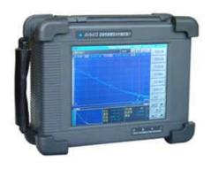
The P5 is a high performance mini-OTDR, which is small in size, light in weight and rugged in configuration. It has a large color LCD and a USB interface. It also features a long battery operation life. With the P5 series OTDR, you can measure unit/connection/transmission loss and locate faults or breaks on optical fibers.
