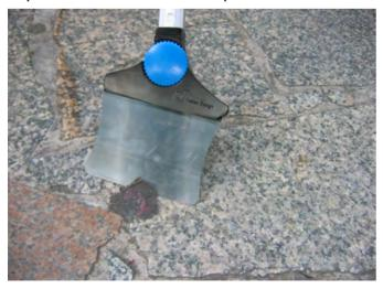
Super blade; blunt edge especially for removing glue and paint on the floor
