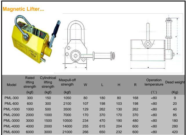
★ Principles:Model PML Permanent Magnet Lifter has strong magnetic path producde by Nd-Fe-B magnetic materials. On and Off of the magnetic path is controlled by turning the manual handle PML permanent magnetic lifters have magnet as power, and its lifting power will never weaken.
