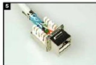
5 Check and ensure each wire in correct channel, tight cable tie at the end of shielded case.
