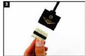
3 4-pair impact tool seats connecting blocks.
