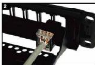
Position the keystone jack for installation.
